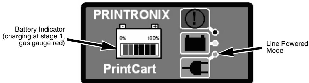
**Figure 12. Operating in Unrestricted, Line Powered Mode**
