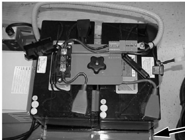
**Figure 19. Power Equipment Subpallet**
